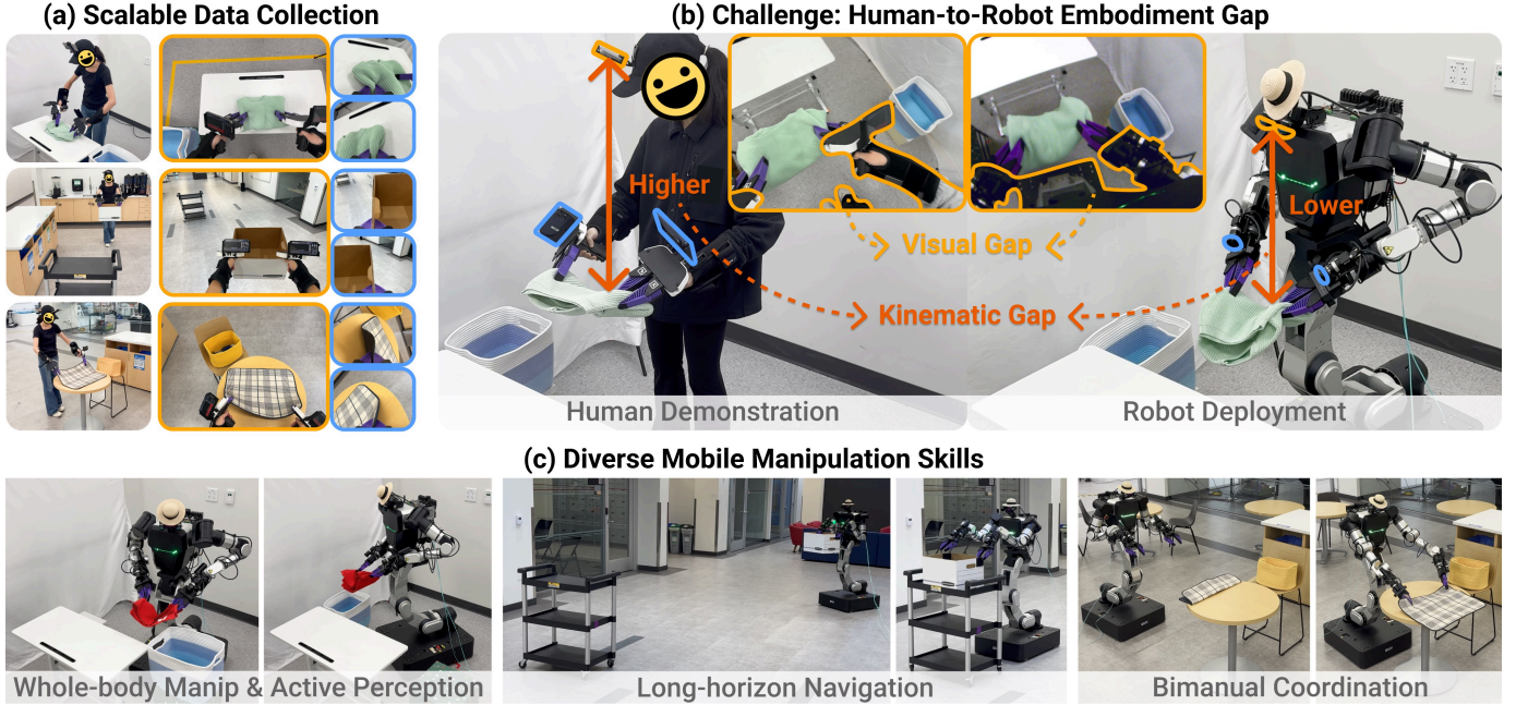
Fig. 1: Whole-Body Mobile Manipulation Interface (HoMMI) . (a) We extend UMI with egocentric sensing to enable scalable mobile manipulation with active perception – capabilities that cannot be achieved with the original UMI. (b) However, the new egocentric view creates a substantial embodiment gap in both observation and action space, making policy transfer difficult. (c) We bridge this embodiment gap by carefully redesigning the visual and action representations and integrating them with a constraint-aware whole-body controller. Together, HoMMI is able to learn diverse mobile manipulation skills directly from human demonstrations, without any robot teleoperation data.
